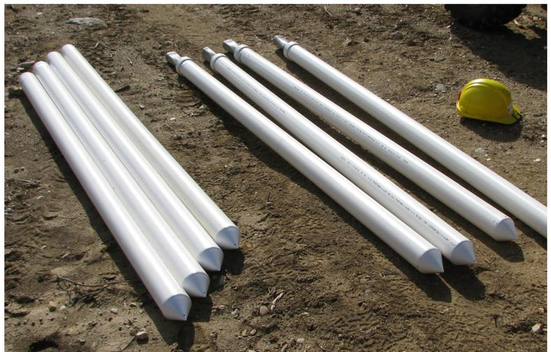
Figure 4. Monitoring wells were made of perforated PVC plastic pipe with conical shaped bottoms. A stretchable fabric sock installed around the pipe (not shown in picture) kept sediment and debris from entering the well through the perforations. Wells had either a removable cap on top to allow for manual water level measurements and sampling (left) or a digital water level recorder as the cap (right).
