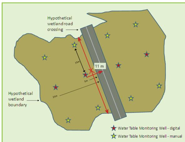
Figure 1. Layout of sampling design showing placement and location of digital and manual water table monitoring wells. Courtesy of Ducks Unlimited Canada.
