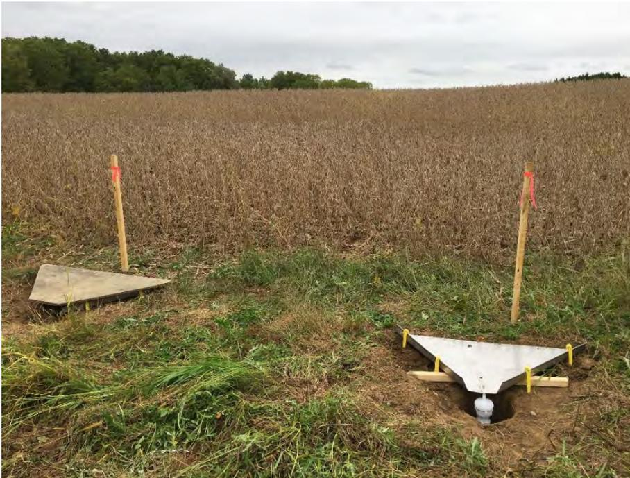
**Figure A 13.** Runoff trays at site DY with protective cover on (left) and off (right) with deployed sample bottle with cover designed to keep dust out of bottle when no flow occurs and to collect runoff water slowly to collect water sample over the runoff period.
