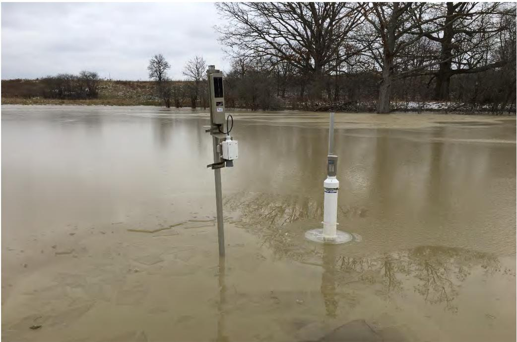
**Figure A 1.** Picture of site OH with ecotone water level recorder and AP3 water level recorder in the foreground.
