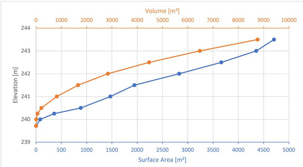
**Figure A 21.** DY storage curve.
