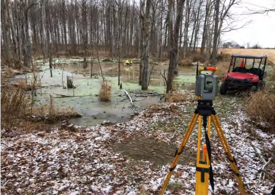
**Figure A 8.** Picture of site MA while basin bathymetry data being collected.
