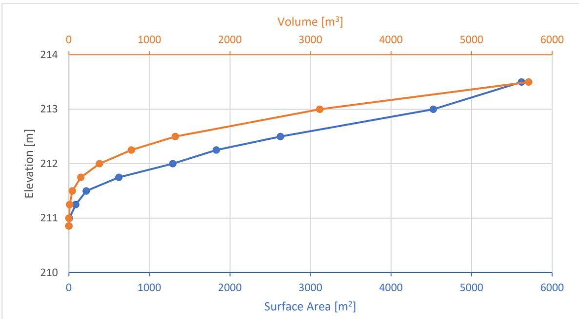
Figure A 17. KE storage curve.
