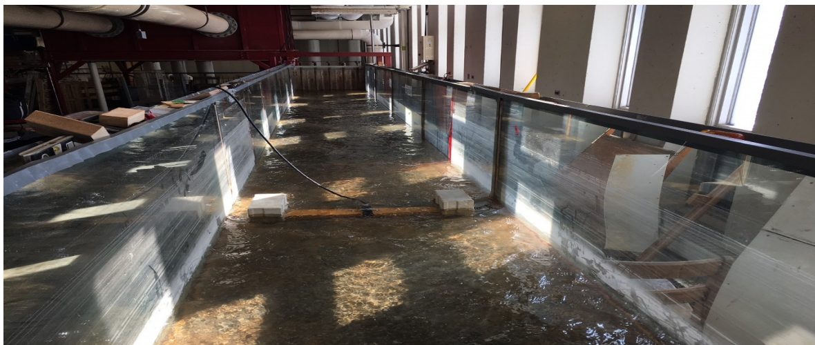
Figure A 9. Picture of an area velocity flow probe being tested for accurate calibration in a controlled flume at the Hydraulics Research and Testing Facility at the University of Manitoba prior to deployment in the field.
