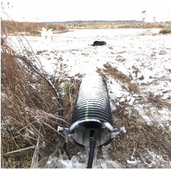
Figure A 10. Deployed area velocity flow probe collecting flow data every 15 minutes at the outflow of site KE.
