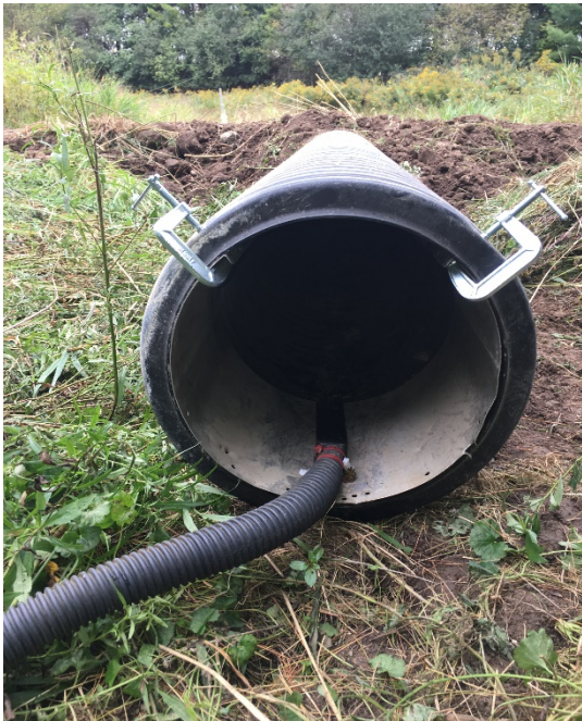
Figure A 11. Close up of area velocity flow probe the outflow of site DY at period when site DY is not spilling.
